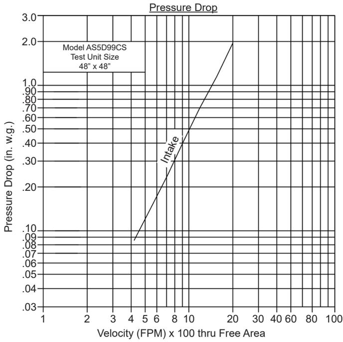
Intake air converted to standard air density.
